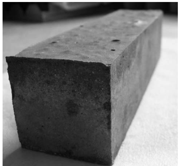
Figure 13. Geopolymeric mortar (4×4×16 cm body) after 600 days of immersion in \text{MgSO}_4 solution.
