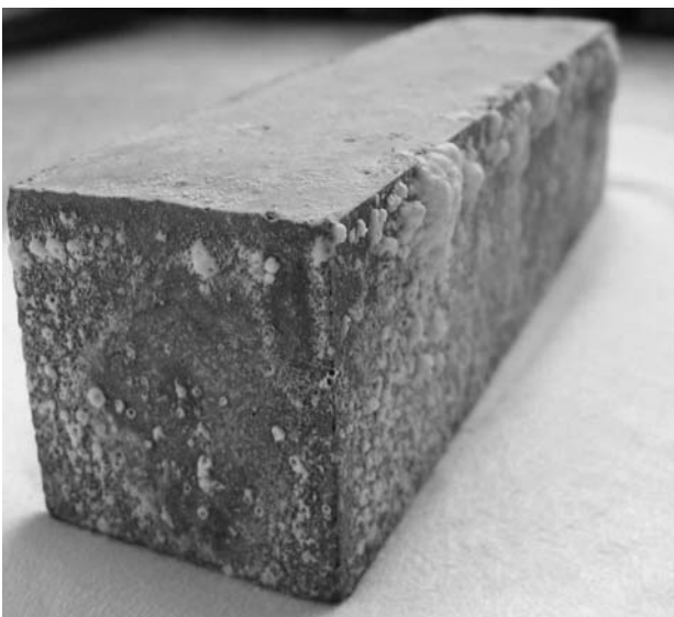
Figure 12. Geopolymeric mortar (4×4×16 cm body) after 600 days of immersion in \text{Na}_2\text{SO}_4 solution.
