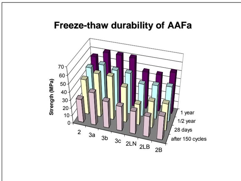
freezing and defrosting cycles in aqueous environment. The mass of the samples did not change (no body disintegration occurred) during the freezing and defrosting cycles in aqueous environment. The values of the compressive strength of samples were smaller after defrosting cycles as compared with the values obtained for the samples after 28 days without any frost resistance
