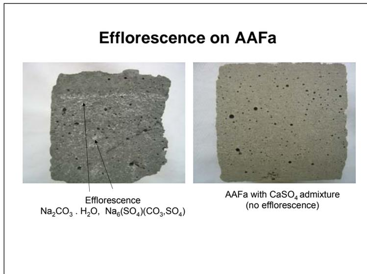
Efflorescences often occurred on the surface of AAFa samples. However, no efflorescences could be seen on fired samples kept (after firing) at the laboratory temperature for 720 days. The efflorescences did not occur on samples treated in this way before their exposure to the aqueous environment. A white coating on the surface of AAFa
