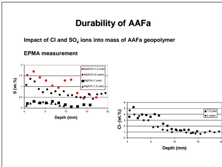
The penetration of sulfate ions into the AAFa body (measured perpendicularly from the surface in contact with the sulfate solution) showed a decreasing tendency; the sulfate concentration in the body was very low. The concentration of sulfate ions during the exposure of the material to the corrosion by MgSO<sub>4</sub> solution was smaller than during its exposure to Na<sub>2</sub>SO<sub>4</sub>,
