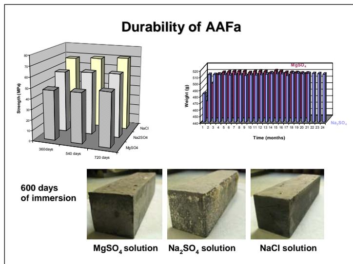
observed. In contrast to Portland cement, no visible damage of samples occurred even if they were kept in corrosive solutions continuously for 720 days.
