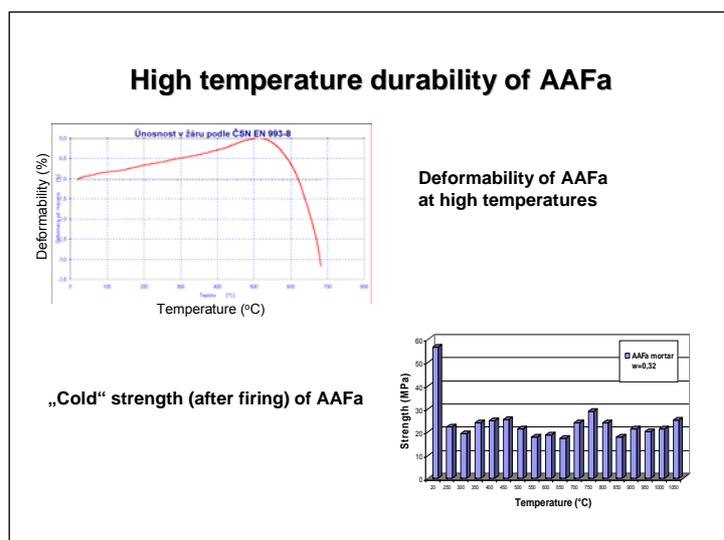
temperature range in which the AAFa body starts softening and the sample dimension subjected to the load force begins to decrease. The  $T_{0.5}$  value was obtained for temperatures ranging from 576 to 589 °C. Therefore, AAFa bodies can not be characterized as purely refractory material.
