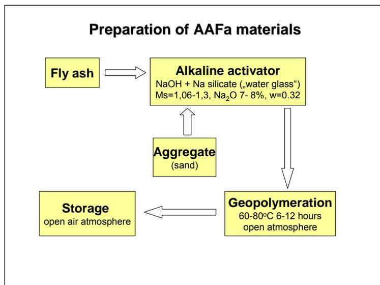
Small bodies having the dimensions of 20 x 20 x 20 mm were prepared from slurries whereas larger samples with the dimensions of 40 x 40 x 160 mm were made from mortars. The bodies prepared in such a way and ready for testing were subjected to a "dry" thermal process that consisted in placing them in a drier (free atmosphere) at a temperature of 60 to 90 °C
