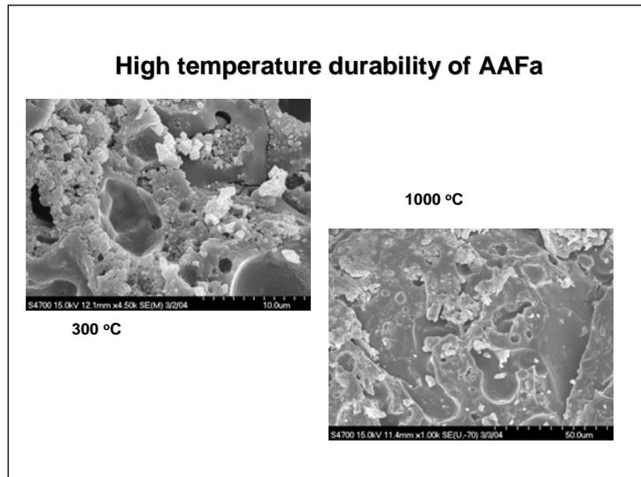
dropped to 40 percent of its original value. The loss of compressive strength becomes already obvious at a temperature of 250 °C and the firing at higher temperatures does not practically affect this parameter. The minimal values of the residual compressive strength were observed in the temperature range of 600 to 700 °C; they were caused by the occurrence of the melt that
