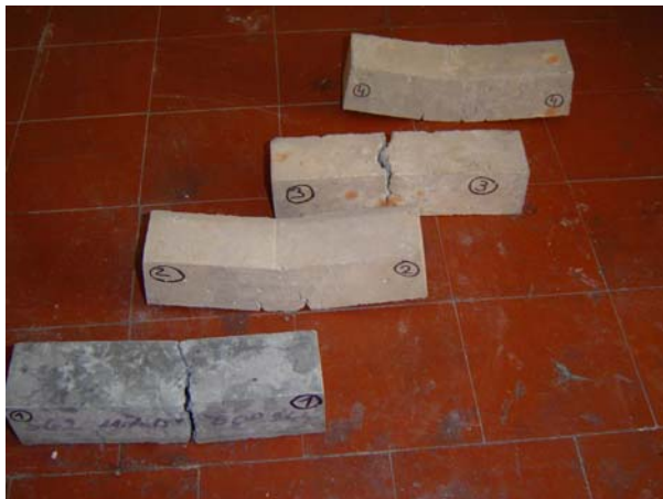
Fig. 27 Deformation character of the geopolymers mortars during the firing
