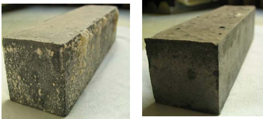
Fig. 25 A geopolymers mortar after the 1.5-year exposure to the solutions of NaCl and \text{MgSO}_4 salts
