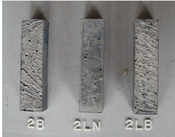
Fig. 24 A geopolymer mortar after 150 freezing cycles
