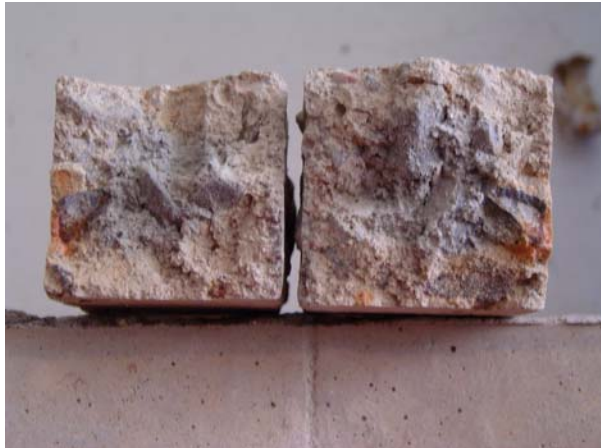
Fig. 26 Character of the geopolymers concrete after firing
