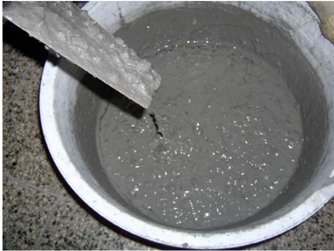
Fig. 3 Character of the fresh geopolymers concrete
