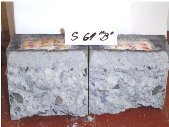
Fig. 4 Incorrect mix, aggregate segregation and the mortar displaced towards the surface
