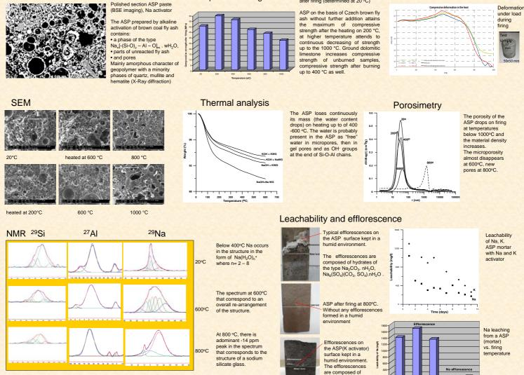
The Na (and K) bond in the ASP structure is weak and this fact explains the tendency of ASP to efflorescences.
