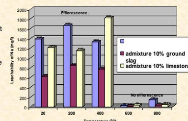
**The Na bond in the geopolymer structure is weak and this fact explains the tendency of geopolymer to efflorescences.** The K leaching from the geopolymer structure is comparable or even larger than that of Na (MacKenzie 2006).
