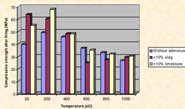
Strength values of the geopolymer (mortar) after firing (determined at 20 °C)
