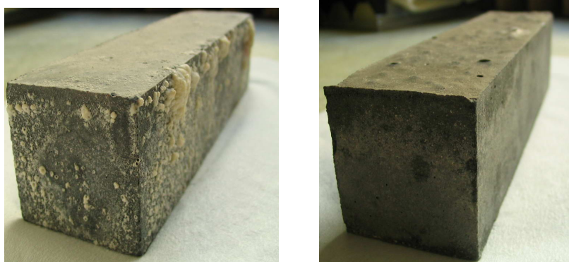
Fig. 25 A geopolymers mortar after the 1.5-year exposure to the solutions of NaCl and MgSO 4 salts
