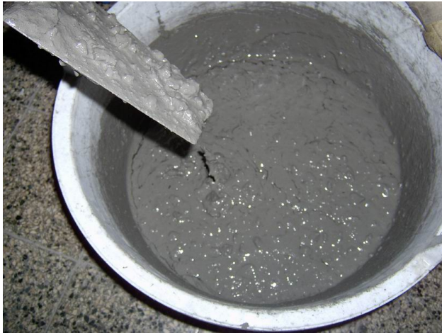
Fig. 3 Character of the fresh geopolymers concrete
