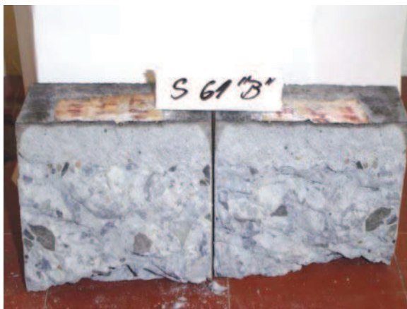
Fig. 4. Incorrect mix, aggregate segregation and the mortar displaced towards the surface.
