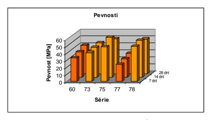
Pct. 1 – Press strength of POPbetonu® - tempered
