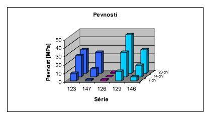
Pct. 2 – Press strength of POPbetonu® - non-tempered
