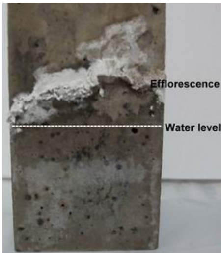
FIG. 9 Typical efflorescences on the geopolymer surface kept in a humid environment. The efflorescences are composed of hydrates of the type \text{Na}_2\text{CO}_3 \cdot n \text{H}_2\text{O} , \text{Na}_6(\text{SO}_4)(\text{CO}_3, \text{SO}_4) \cdot n \text{H}_2\text{O} .
