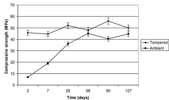
Fig. 8 Compressive strength of “tempered” and “ambient” concrete vs. time (fly ash content in the mixture 400 kg/m<sup>3</sup>).
