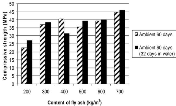
Fig. 10 Compressive strength of "ambient" concrete.
