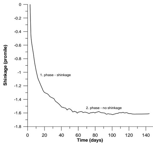
Fig. 15 Shrinkage of concrete "ambient".
