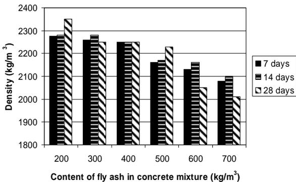
Fig. 12 Density of concrete ("ambient").
