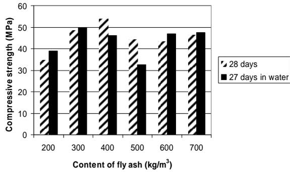
Fig. 9 Compressive strength of "tempered" concrete.
