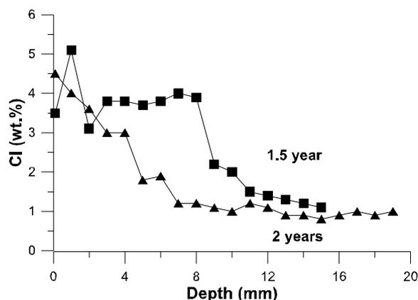
**Fig. 19** Penetration of Cl<sup>-</sup> (measured as Cl) in alumosilicate polymer concrete (1.5 years in NaCl solution), point analysis.
