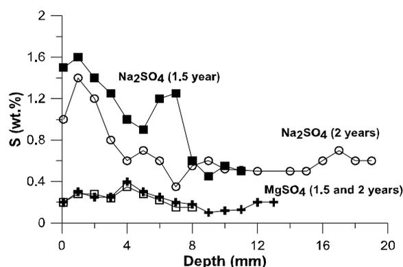
**Fig. 20** Penetration of SO<sub>4</sub><sup>2-</sup> (measured as S) in alumosilicate polymer concrete (1.5 years in Na<sub>2</sub>SO<sub>4</sub>, MgSO<sub>4</sub> solution), point analysis.
