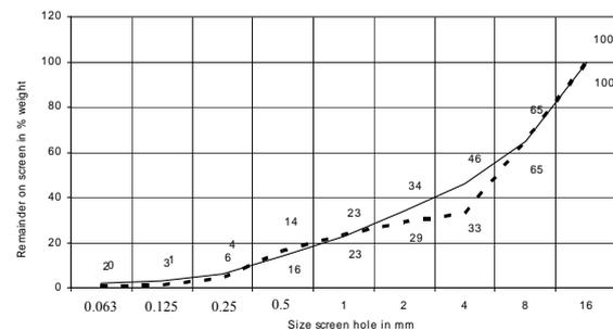
**Fig. 2** Spline aggregate gradation 0/4, 4/8, 8/16 in comparing to exemplary spline.
