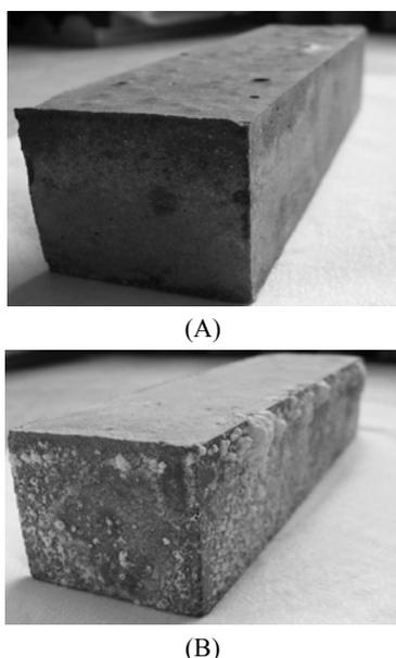
**Fig. 18** Alumosilicate polymer concrete after the 1.5-year exposure to the solutions of NaCl (A) and MgSO<sub>4</sub> (B) salts.
