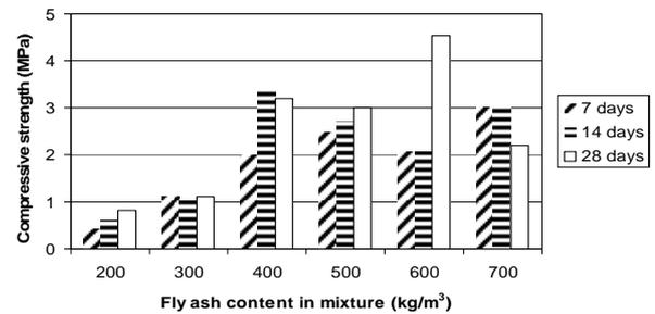
Fig. 14 Compressive strength of concrete, at -20 °C.
