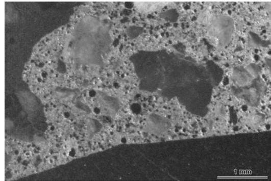
Fig. 7 Alumosilicate polymer concrete (polished section, optical microscope).
