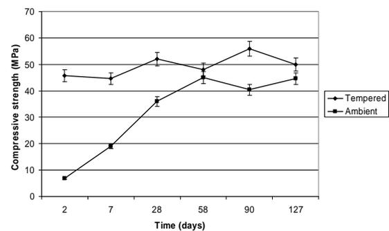
Fig. 8 Compressive strength of “tempered” and “ambient” concrete vs. time (fly ash content in the mixture  $400 \text{ kg/m}^3$ ).
