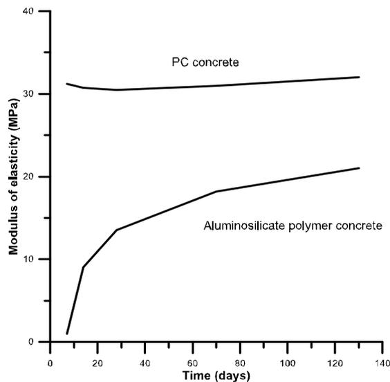
Fig. 16 Modulus of elasticity vs. time.
