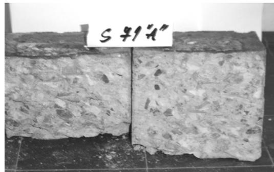
Fig. 5 Correctly composed mix, uniform distribution of the aggregate.
