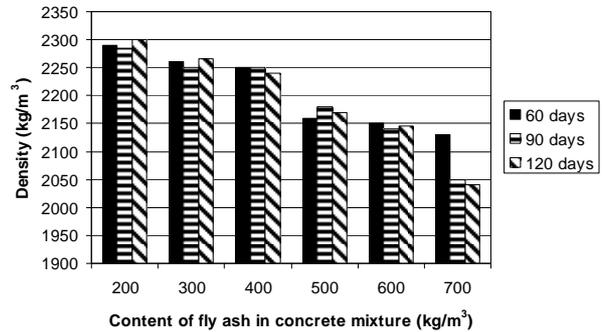
Fig. 13 Density of concrete ("tempered").
