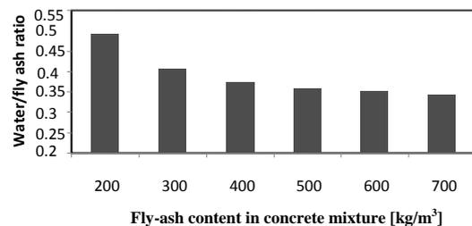
**Fig. 3** Water to fly ash vs. fly ash content in concrete mixture at same workability (S3 slump test).
