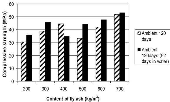
Fig. 11 Compressive strength of "ambient" concrete.
