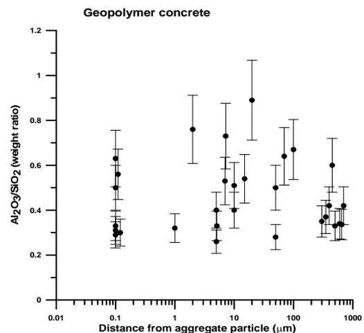
Fig. 17 Dependence of the  $\text{Al}_2\text{O}_3$ -to- $\text{SiO}_2$  ratio on the distance from the aggregate grain in a aluminosilicate polymer concrete.
