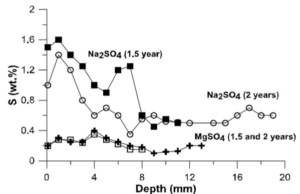
**Fig. 20** Penetration of SO<sub>4</sub><sup>2-</sup> (measured as S) in alumosilicate polymer concrete (1.5 years in Na<sub>2</sub>SO<sub>4</sub>, MgSO<sub>4</sub> solution), point analysis.
