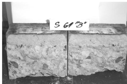
Fig. 6 Incorrect mix, aggregate segregation and the mortar displaced towards the surface.
