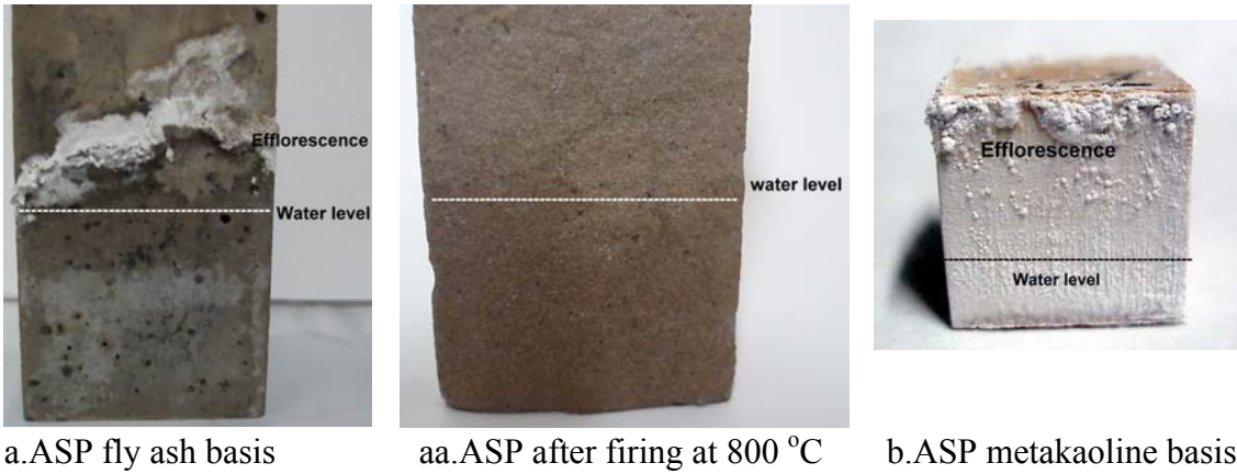
Fig.8 Efflorescences on the ASP (Na activator) surface kept in a humid environment. The efflorescences are composed of hydrates of the type \text{Na}_2\text{CO}_3 \cdot n \text{H}_2\text{O} , \text{NaHCO}_3 \cdot n \text{H}_2\text{O} , seldom \text{Na}_6(\text{SO}_4)(\text{CO}_3, \text{SO}_4) \cdot n \text{H}_2\text{O} .
